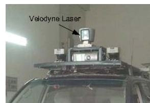
Figure 1. Autonomous vehicle used in this paper, equipped with Velodyne HDL-64E S2 Laser.
