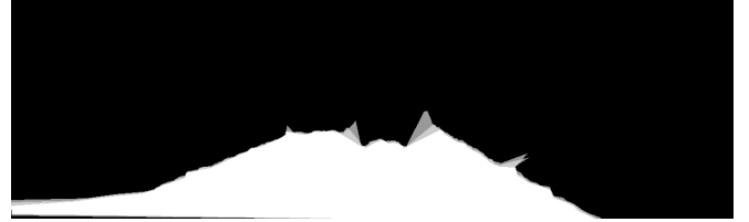
Fig. 3. Result of our road estimation method as confidence map to Fig. 2. The combination of several histograms improves classification results in road border area.
