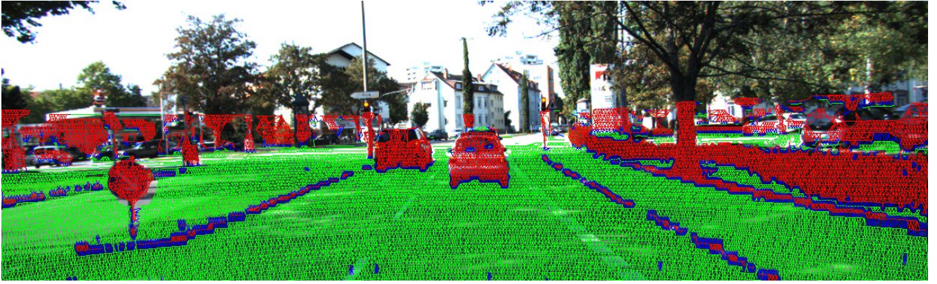
Fig. 1. Results from our obstacle detection method in 2D image world. Red represents edges between two points classified as obstacle , green represents edges between non-obstacles points, and blue represents edges between non-obstacle points and obstacle points.
