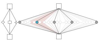
Figure 1. Search space comparison between searching for network architecture and receptive field combinations. Left: Network architecture search mostly search for several operations with different functions. Right: The search space of receptive field combinations is huge. The white, gray, blue nodes and red shade represent the dilation rate candidates, the sparse search space in global search, one of the global searched results, and the local search space.
