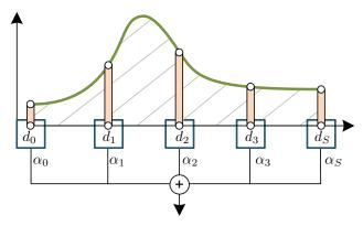
Figure 4. The approximated probability mass function of dilation rates is determined by the multi-dilated convolutional layer with shared weights.
