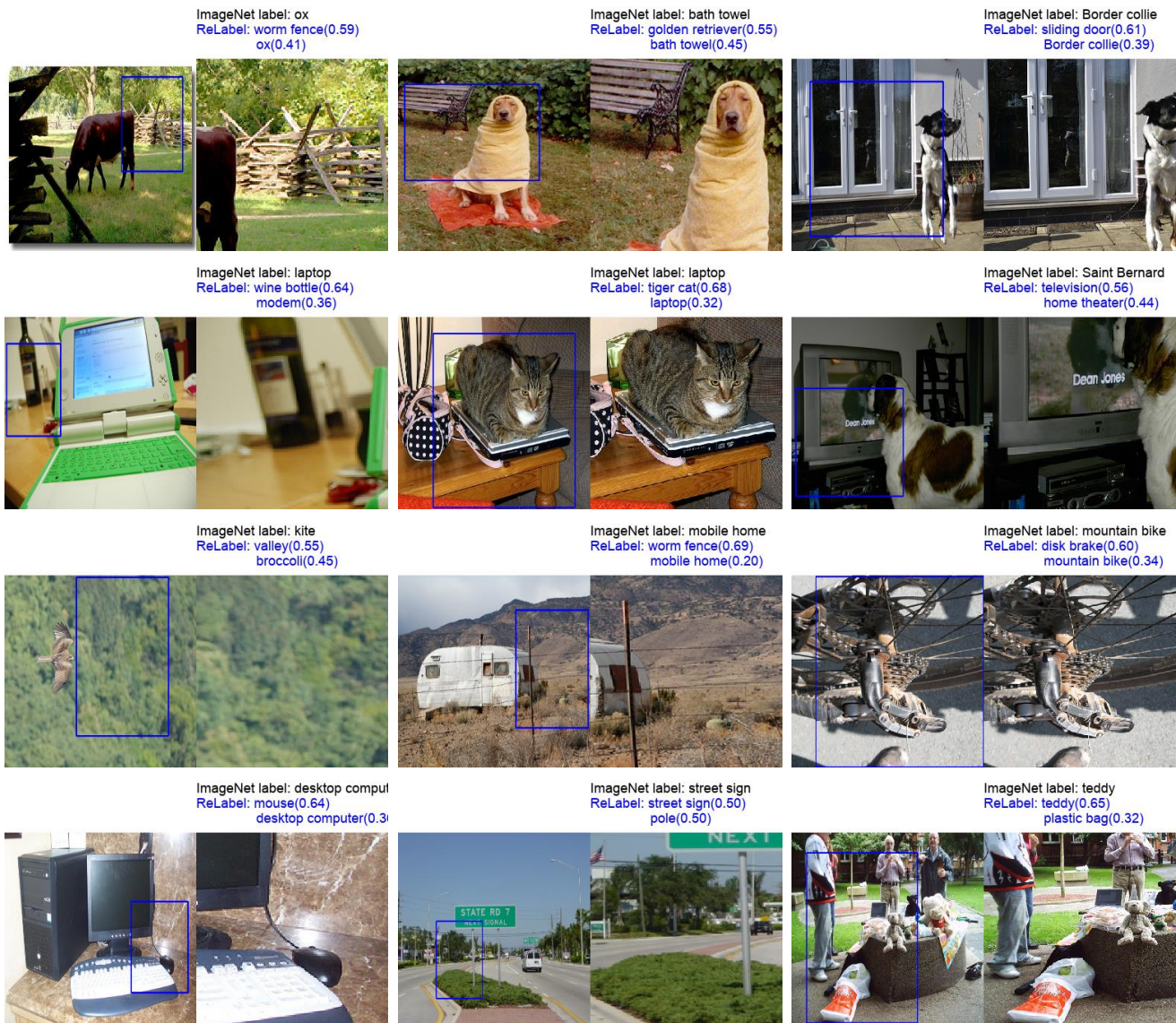
Figure A3. ReLabel examples during ImageNet training. We present selected examples generated by ReLabel during ImageNet training. For each example, the left image is the full training image and the right image is the random cropped patch. The random crop coordinates are denoted by blue bounding boxes. The original ImageNet label and ReLabel are also presented.
